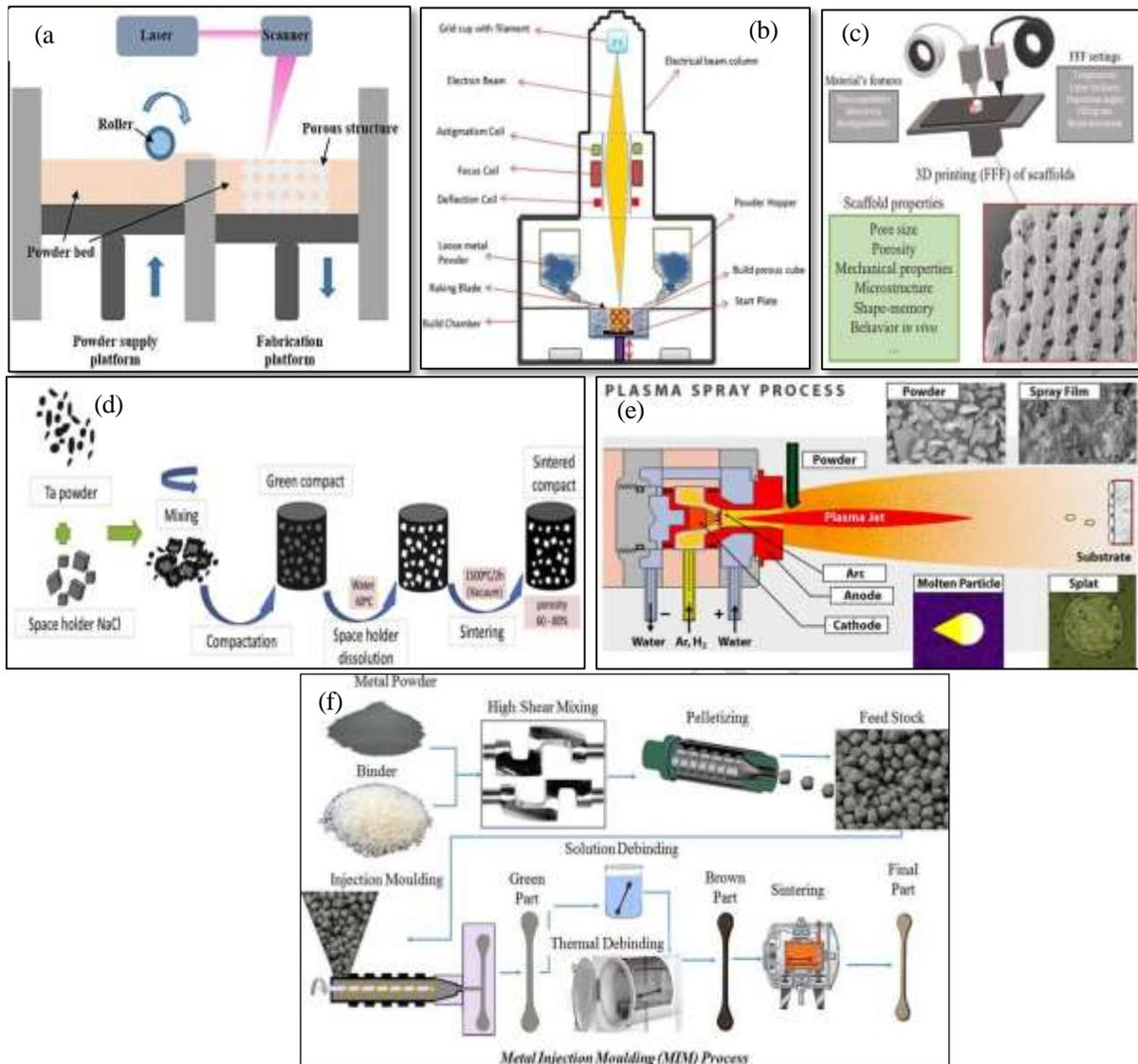
Fig. 5 Illustration depicting the principals of: (a) selective laser sintering and selective laser melting [90], (b) electron beam melting [91], (c) fused filament fabrication (FFF) [92] (d) powder metallurgy [93], (e) plasma spraying [94], and (f) metal injection molding (MIM) [95].
