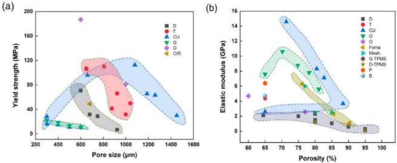
Fig. 4 Correlation between pore size and mechanical properties [74]: (a) Relationship between pore size and yield strength. (b) Influence of porosity on elastic modulus. The symbols denote the lattice structure shapes, such as Diamond (D), Gyroid (G), Primitive (P), and Cube (C). TPMS stands for triply periodic minimal surface [74].
