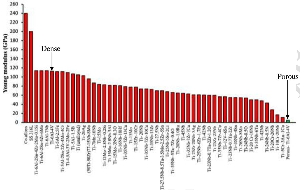
Fig. 2 Elasticity modulus of various dense titanium alloys with a comparison of porous Ti-6Al-4V.
