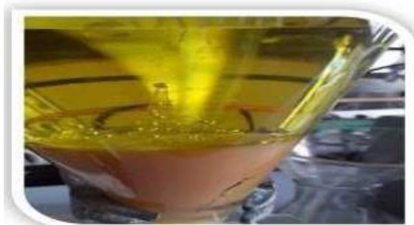
**Photo 2.** Oily and aqueous two phases of *Silybum marianum* ethanol-hexane extract in a separating funnel.
