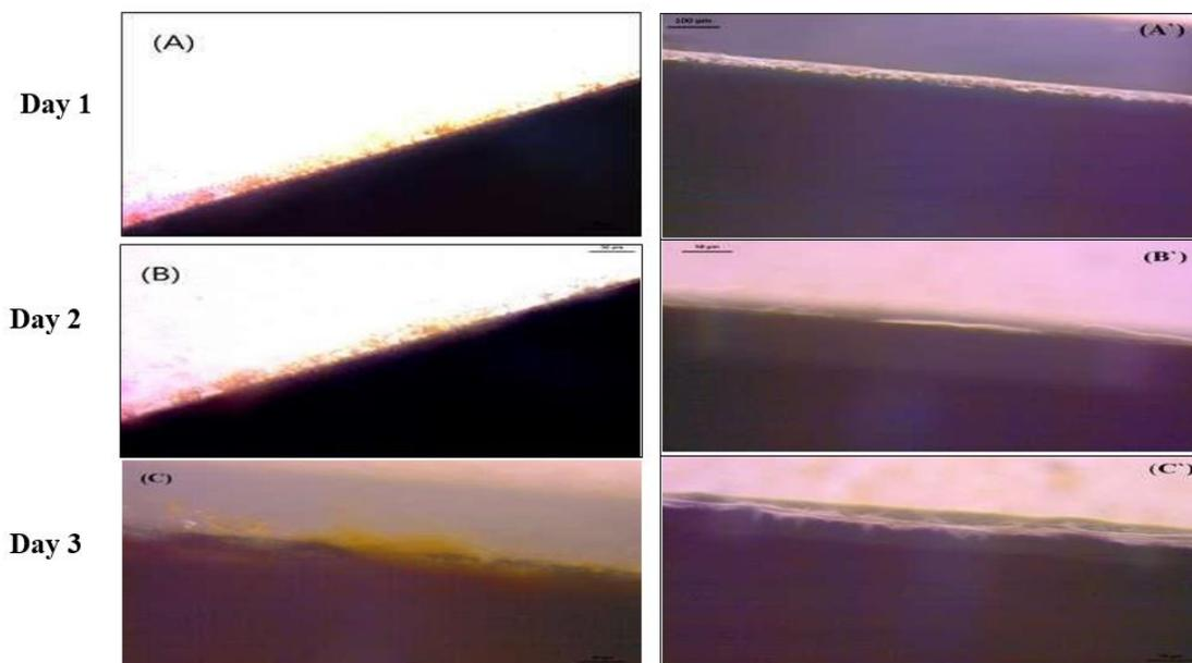
**Photo 3.** Optical microscopic images of the iron metal surface over three successive days A, B, C immersed in fresh water as control and A', B', C' immersed in *S. marianum* ethanol-hexane crude extract as treated.
