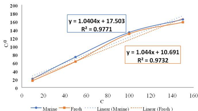
**Figure 2.** Langmuir adsorption isotherm plot for the adsorption of *S. marianum* ethanol-hexane crude extract on the iron metal surface.
